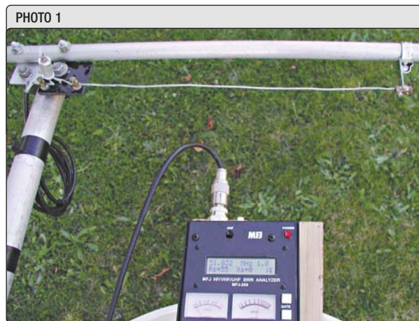
Photo 1 Gamma match on a 50MHz two-element beam using 14SWG copper wire as the gamma rod. Gamma rod reactance is cancelled with a Philips variable trimmer capacitor. Note the low SWR reading on the MFJ.
