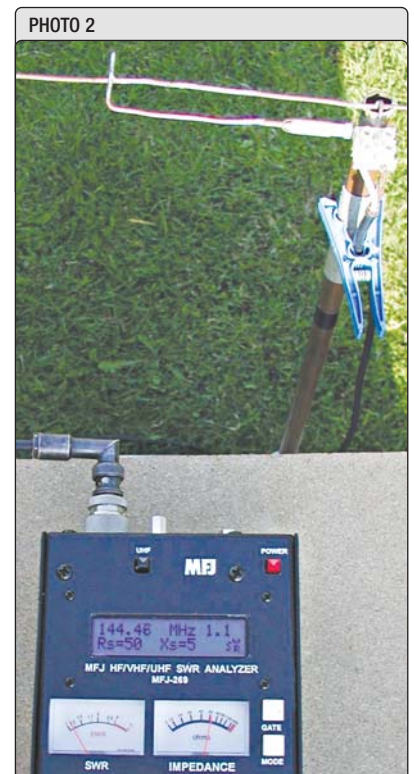
Photo 2 144MHz dipole constructed from 14SWG copper wire and using a gamma rod of the same material. The centre of the dipole element is soldered to the copper tube mast. A concentric ('beehive') trimmer capacitor is used for gamma rod reactance correction.
